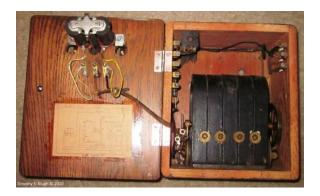
Inside my telephone ringer box is the cool stuff that made it work (even a schematic.) The ringer had a magneto generator (the big black thing on the right side) that would power the electromagnetically-driven hammer (top left) that would rapidly move a ball hammer between the two external ringer gongs.
